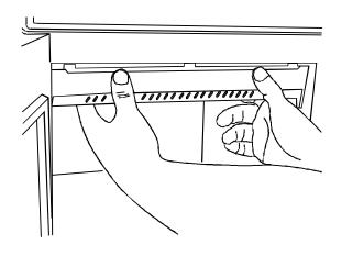
Removing Splatter Shield
